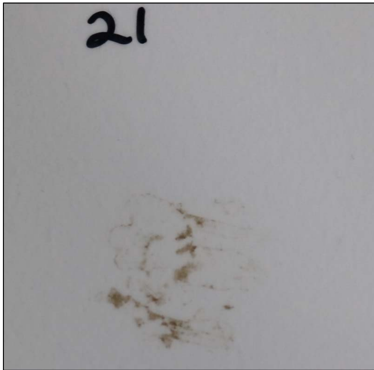
Chemical Spot Test #21, Furfural, Rating 2, Staining
