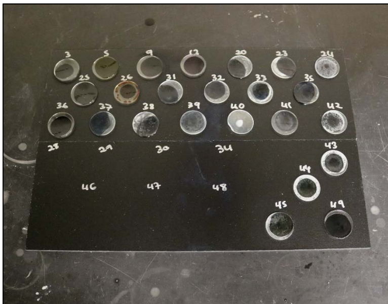
Representative Chemical Spot Test Non-volatile Chemical Set-up
