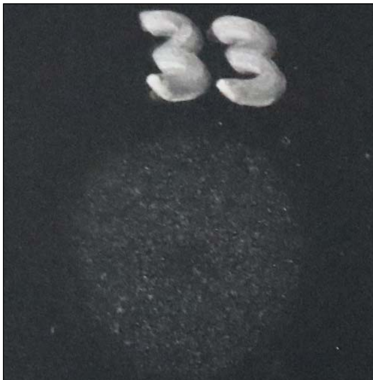
Chemical spot test #33, Nitric Acid (70%), Rating 2, Gloss change
