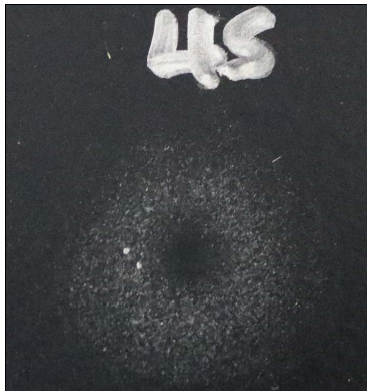
Chemical spot test #45, Sulfuric Acid (77%) and Nitric Acid (70%), equal parts, Rating 2, Gloss change
